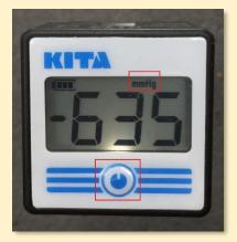
• A normal vacuum level should be between -600 mmHg to -650 mmHg and higher. If the showing units are not mmHg (e.g. kPa, psi or bar) please contact us
